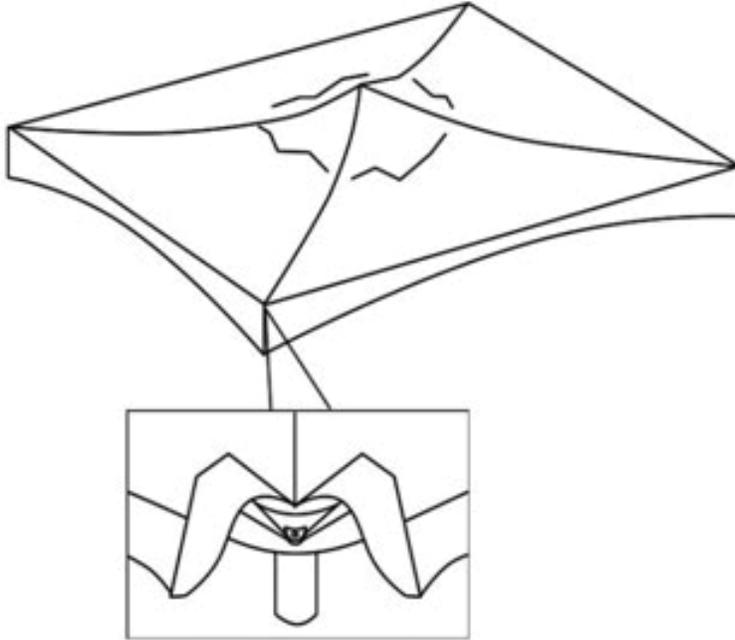
**Step 5:** Assembly the roof cover, pull the corner with handle.
